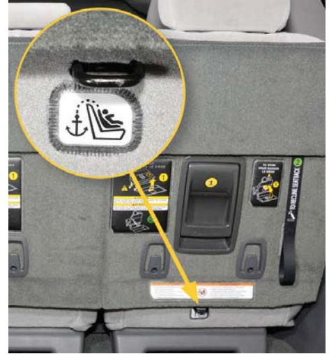
New label added near tether anchor in the 2016 Toyota Sienna for easier identification
